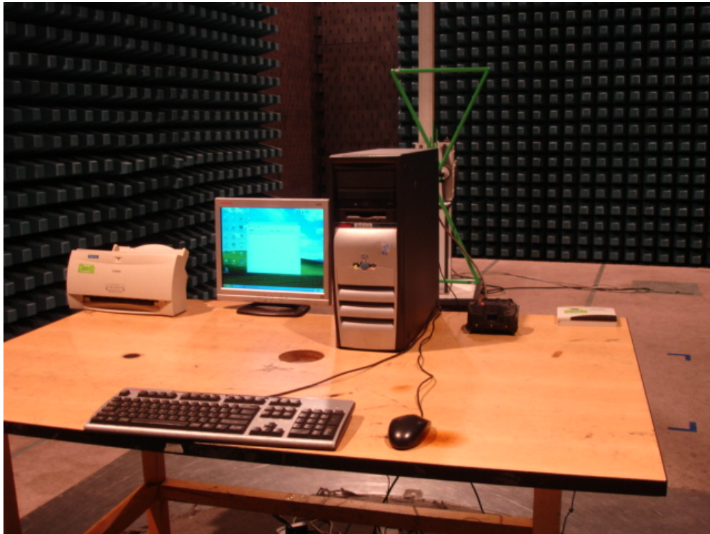
Photo 6 Radiated Emission Test
