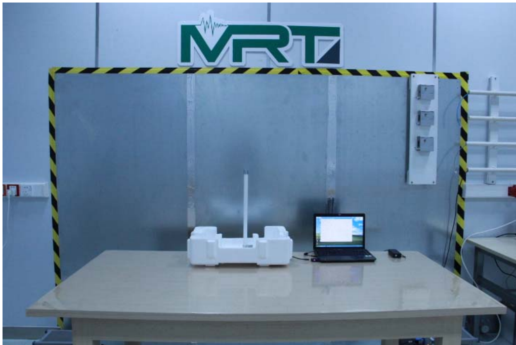
Description: Front view of Conducted Emission Test Setup(With Antenna AO-24008.1)
