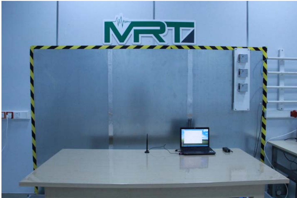
Description: Front view of Conducted Emission Test Setup(With Antenna A-2409D)
