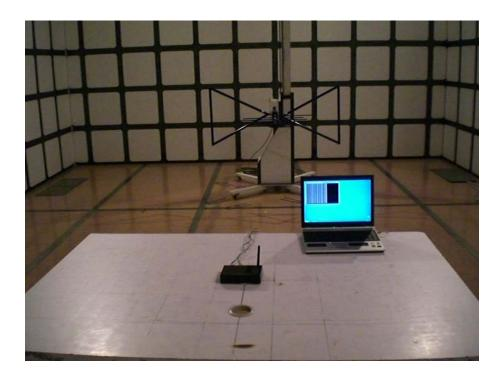
Radiation Emission Test Setup (Above 1GHz)
