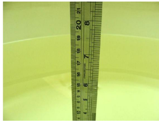
Fig 5.2 Photo of Liquid Height for Body SAR
