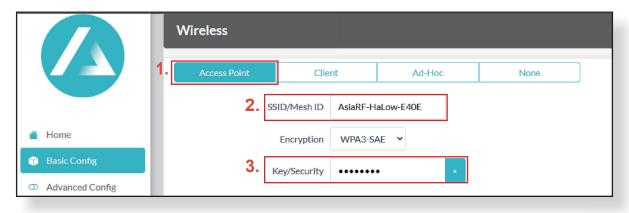
Remember, our default IP address is "192.168.3.3" with the default Wi-Fi- 2.4 GHz SSID being "AsiaRF-WiFi-xxxx" and the password "12345678".
