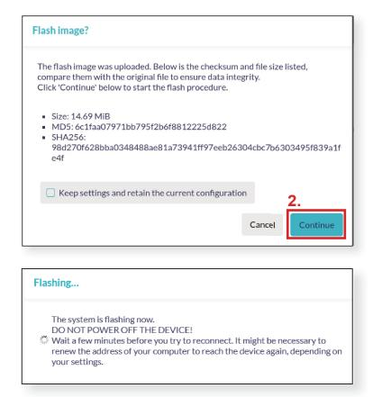
Once the flashing process on the screen completes, the device will automatically restart. Please refer to section 2.2 for guidance on the indicator lights during boot-up. The reboot process usually takes about four minutes.
