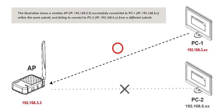
241 Setting a Static IP on a Windows PC for HaLow Gateway Access:
