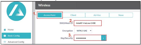
Remember, our default IP address is "192.168.3.3" with the default Wi-Fi- 2.4 GHz SSID being "AsiaRF-WiFi-xxxx" and the password "12345678".
