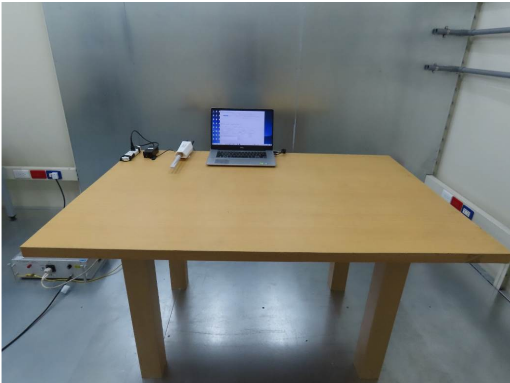
Set Up Photo of Conducted Emission Model No.: ARFHL-OD-MS01
