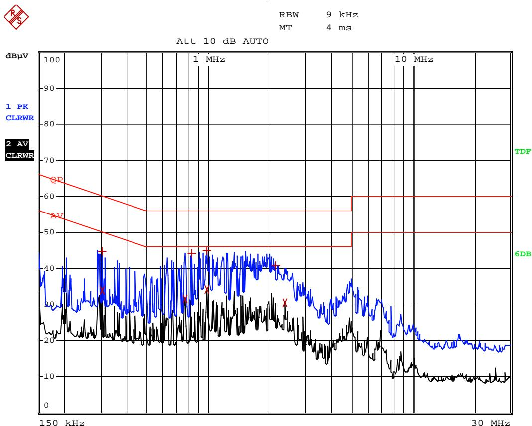
**Plot of Conducted Emissions Test Data***Conducted Disturbance**EUT: 802.11b/g 500mW WiFi Booster**M/N: AIB1105G**Operating Condition: Operating**Test Specification: L**Comment: AC 120V/60Hz XSS Adapter DC 5V*
