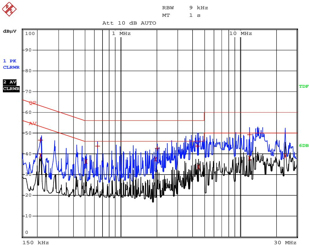
**Plot of Conducted Emissions Test Data***Conducted Disturbance**EUT: 802.11b/g 500mW WiFi Booster**M/N: AIB1105G**Operating Condition: Operating**Test Specification: N**Comment: AC 120V/60Hz XSS Adapter DC 5V*
