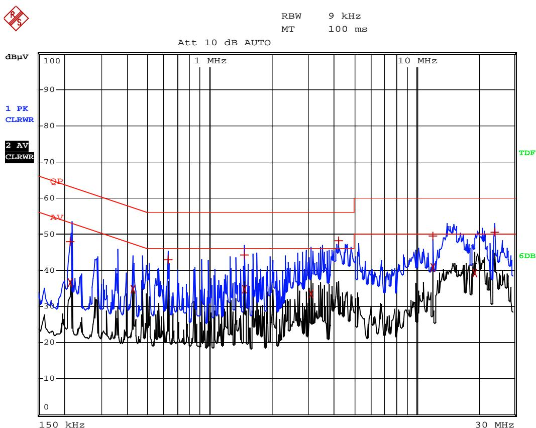
**Plot of Conducted Emissions Test Data***Conducted Disturbance**EUT: 802.11b/g 500mW WiFi Booster**M/N: AIB1105G**Operating Condition: Operating**Test Specification: L**Comment: AC 120V/60Hz TW Adapter DC 5V*
