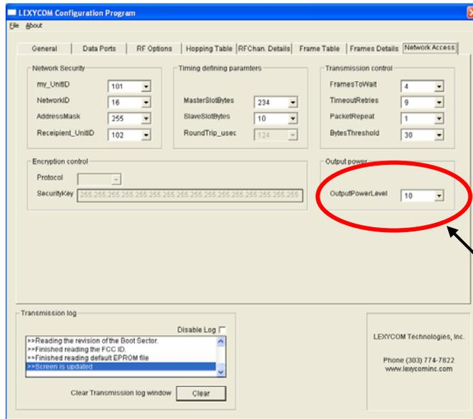
Locate the OutputPowerLevel menu item (shown on the picture above). Click on it and select the desired output power settings.
