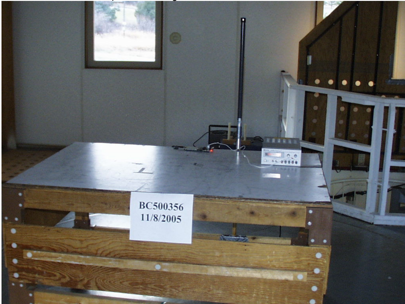
Test-setup photo(s): Radiated Emissions: Sample1 with 5dB gain rod antenna.
