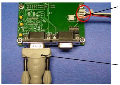
**WARNING:** Polarity of this connector is very important!
