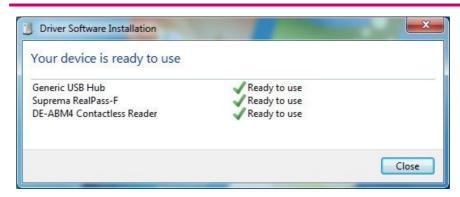
Connect the device's USB cable to a PC and Driver is installed automatically.
