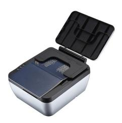
RealPass-F provides full-page, one-step reading of visual data page and RF chip data of ICAO standard passports. For high-level security in immigration clearance, RealPass-F. Sealed in IP54 rated rugged structure, the device features USB 2.0 power and data transfer interface. RealPass-F is an ideal all-in-one device to read
