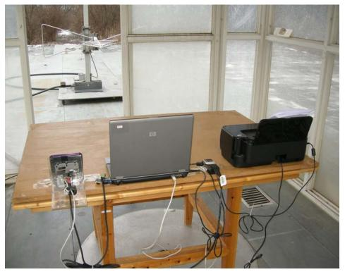
3. Radiated Emission setup : Above 1 GHz (Test Mode : Adapter)
