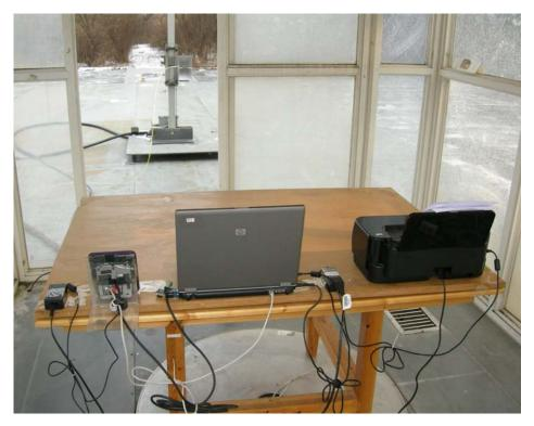
4. Radiated Emission setup : Above 1 GHz (Test Mode : PoE)
