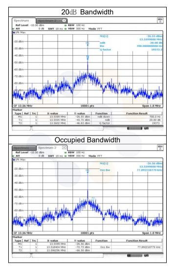
Because the measured signal is CW/CW-like, adjusting the RBW per C63.10 would not be practical since measured bandwidth will always follow the RBW and the result will be approximately twice the **RBW**
