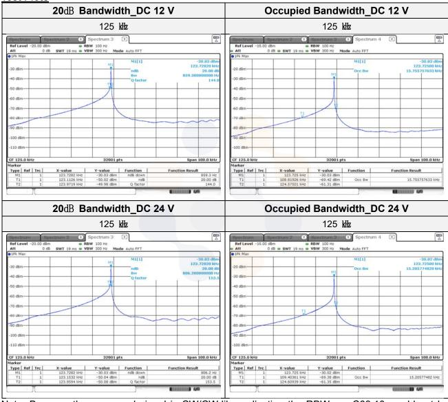
Note. Because the measured signal is CW/CW-like, adjusting the RBW per C63.10 would not be practical since measured bandwidth will always follow the RBW and the result will be approximately twice the RBW.
