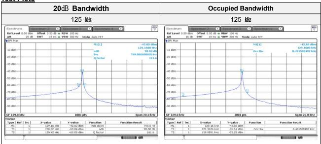
Note. Because the measured signal is CW/CW-like, adjusting the RBW per C63.10 would not be practical since measured bandwidth will always follow the RBW and the result will be approximately twice the RBW.
