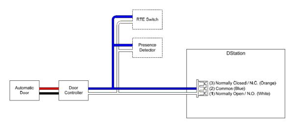
TTL Input Port Connection-RTE Switches
