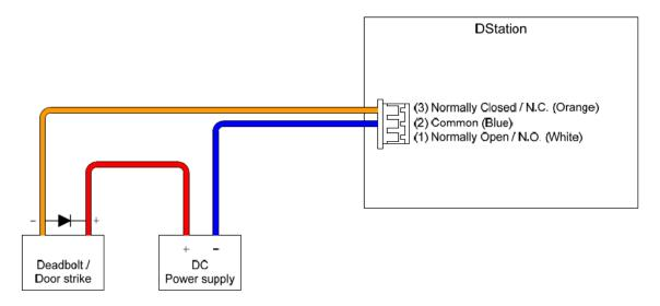
Relay Connection-Fail Secure Lock
