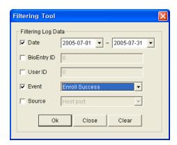
This tool makes it possible to select log data by a field or condition separately.
