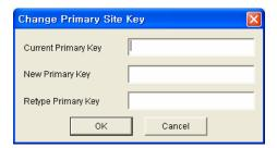
• Each site key can have an integer value from 0 to 281,474,976,710,655. If the input box of primary key remains blank, the default primary site key, 281,474,976,710,655, is input automatically.
