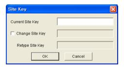
Write – Save the information displayed in the current form to smartcard. If site key has not been input from startup of program, site key can be changed and saved. If writing is stopped by external problems or some other factors in the writing process, the corresponding smartcard is not likely to be used any more - especially while changing site key.
