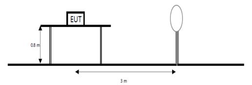
The diagram below shows the test setup that is utilized to make the measurements for emission from 30 Mb to 1 GHz emissions.
