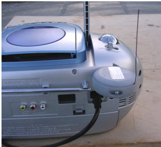
Figure 6: Measurement Test Set-up showing EUT Attached to CD Player
