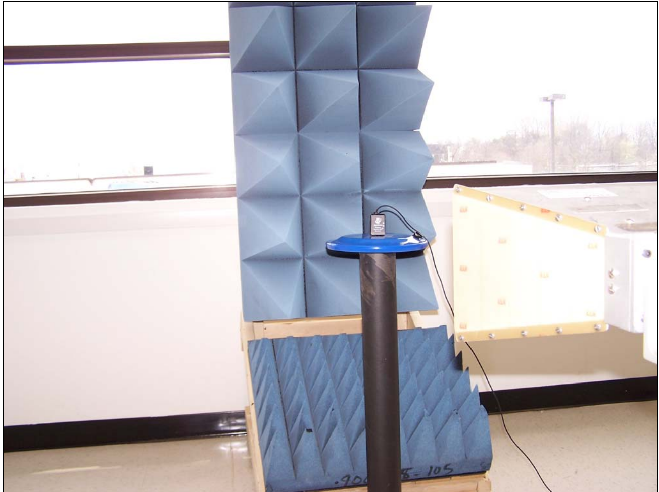
Photograph 2. Radiated Emissions Test Setup, IC3 Receiver
