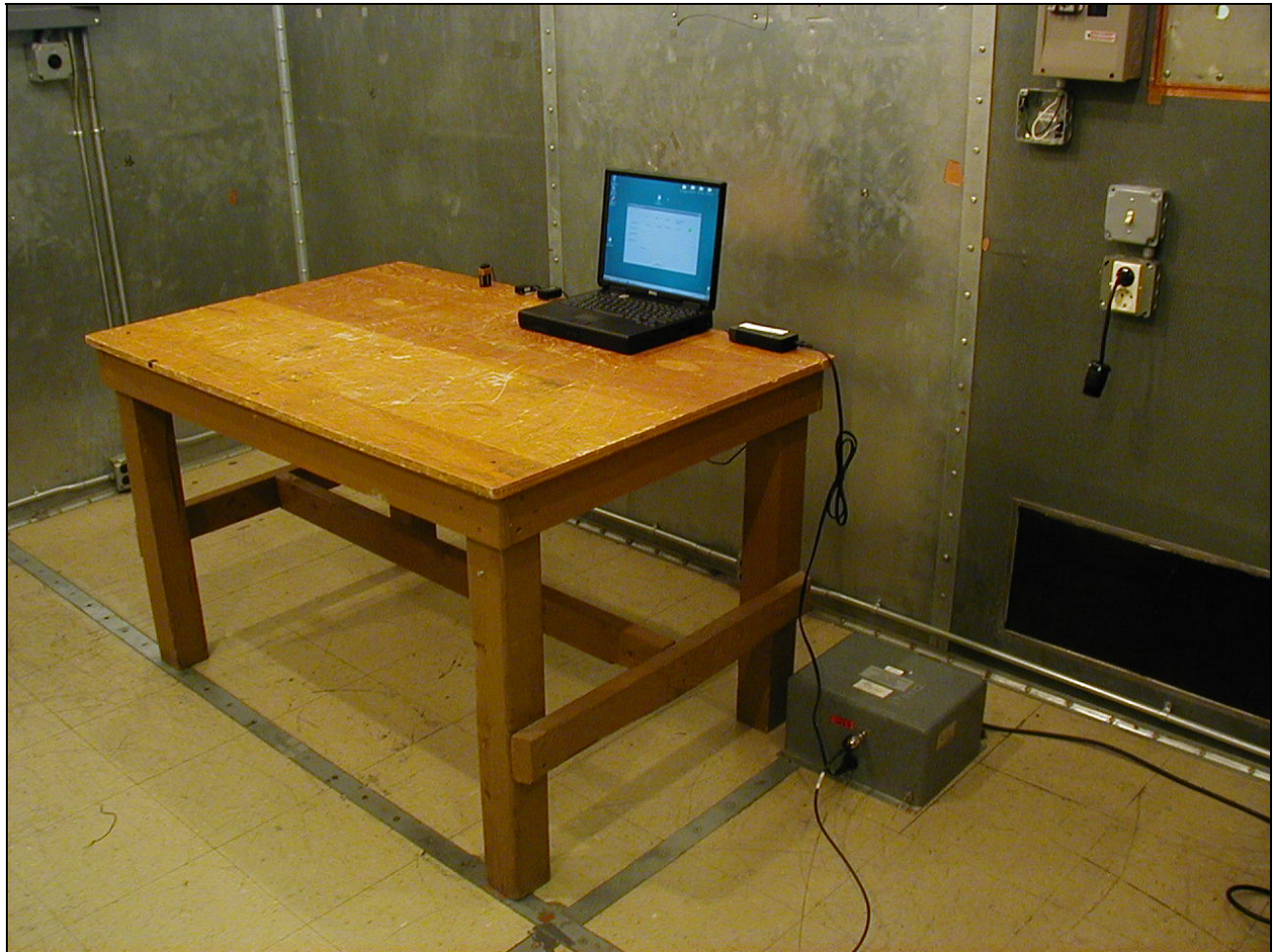
Photograph 3. Conducted Emissions, USB Test Setup
