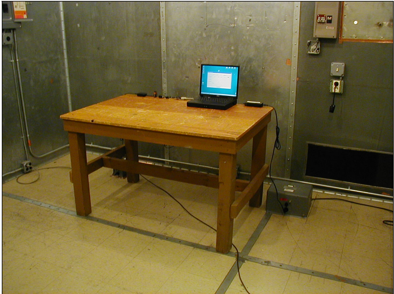
Photograph 4. Conducted Emissions, Serial Test Setup
