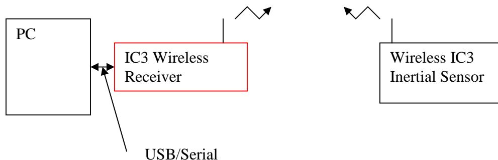
The system is used to detect the orientation of an object that the remote inertial sensor is attached to. The sensor uses gyros, accelerometers and magnetometers to detect its yaw, pitch and roll. Typical uses are for sports training, virtual reality applications and simulation and training.
