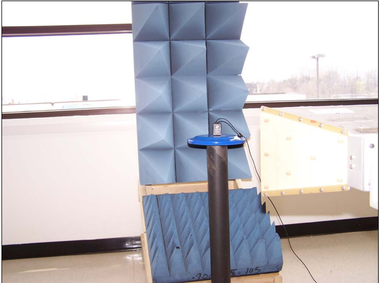
Photograph 2. Radiated Emissions Test Setup, IC3 Receiver
