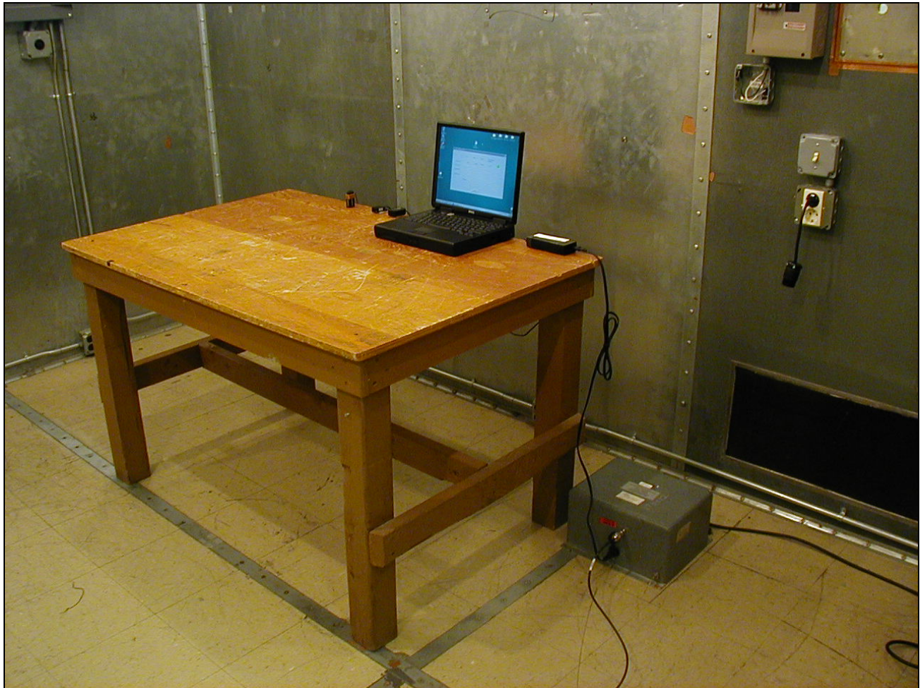
Photograph 3. Conducted Emissions, USB Test Setup
