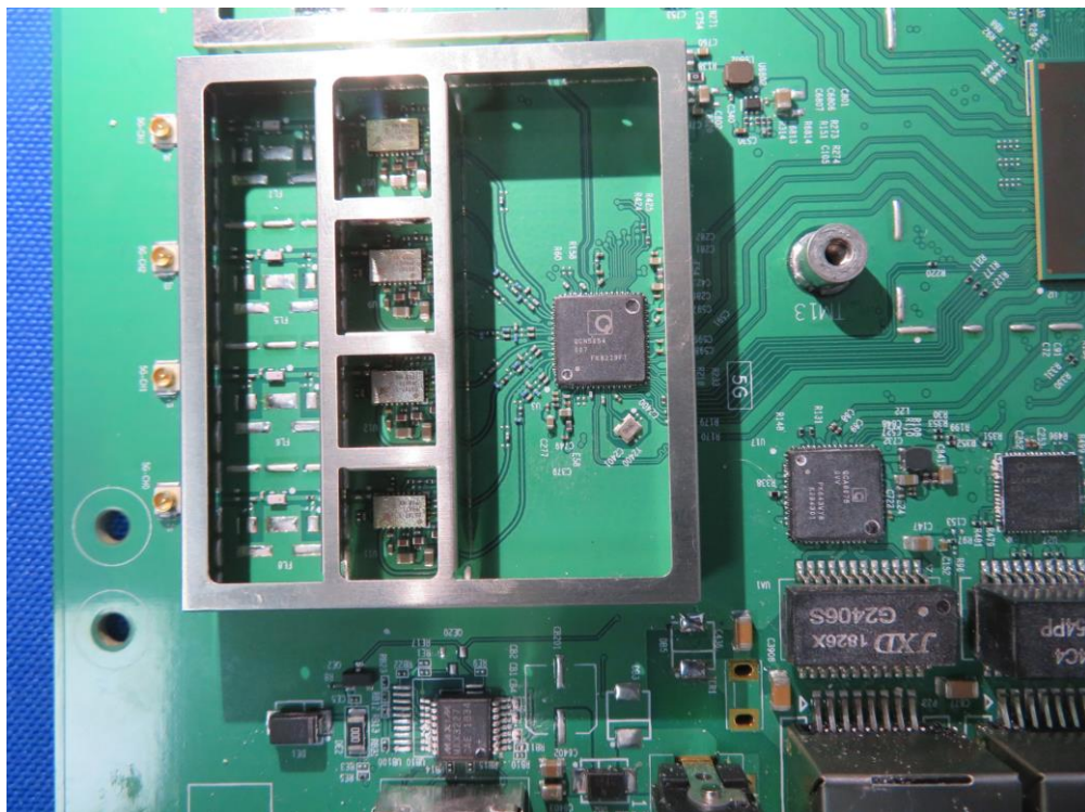
(28) EUT Photo (4x4 Indoor 11ax AP with External SMA Connector)
