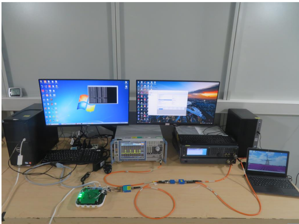
Description: DFS Test Setup
