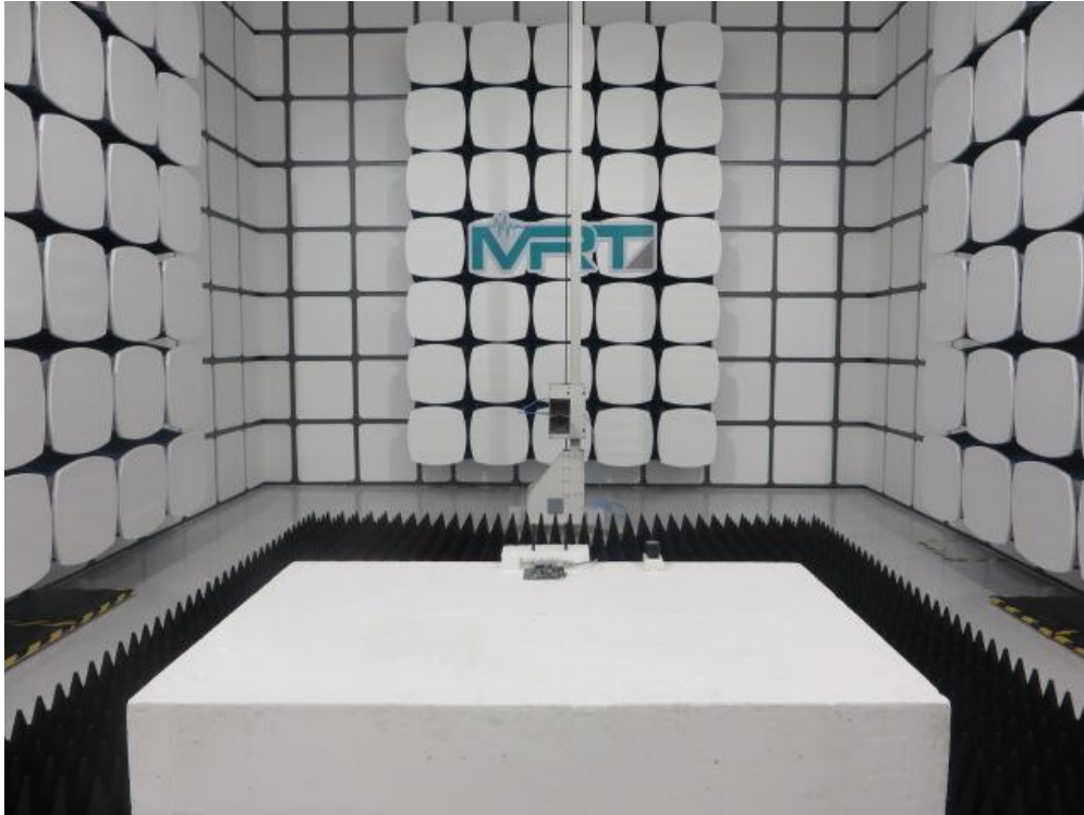
Description: Radiated Emission Test Setup for 18GHz ~ 40GHz (Dipole Antenna 1#)
