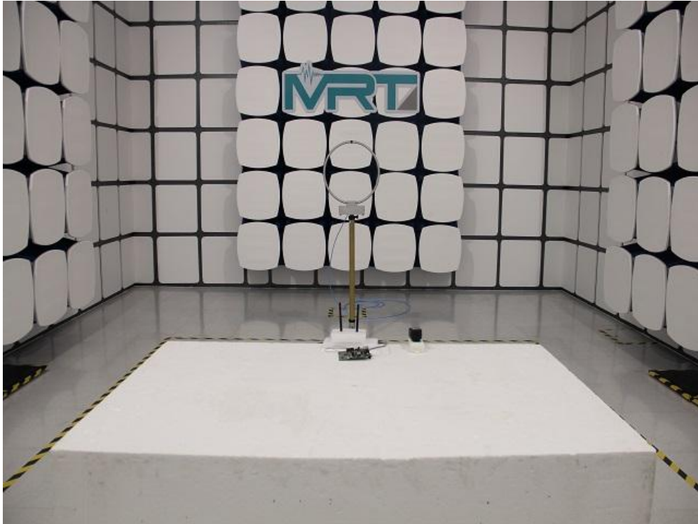
Description: Radiated Emission Test Setup for 30MHz ~ 1GHz (Dipole Antenna 1#)
