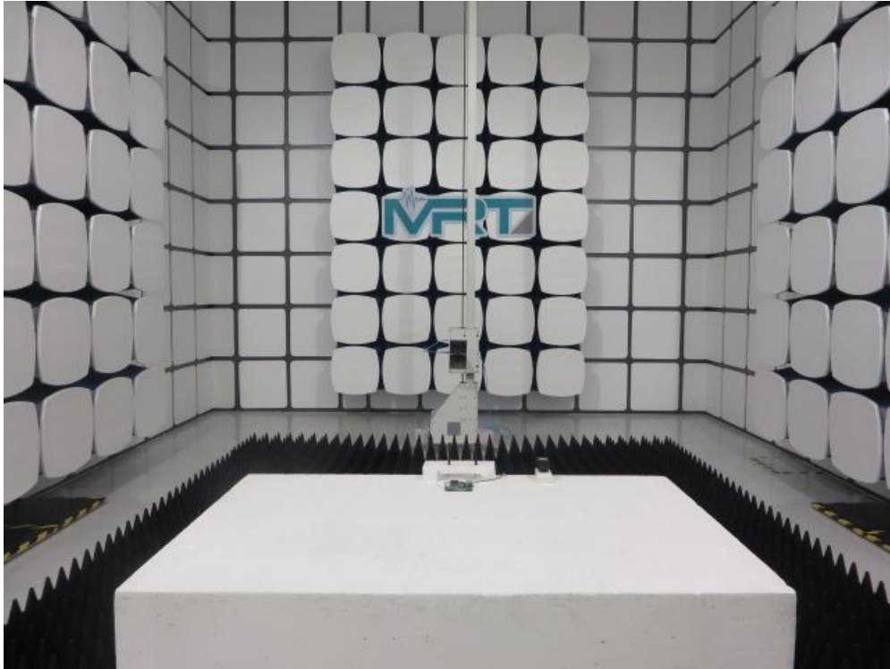
Description: Radiated Emission Test Setup for 18GHz ~ 40GHz (Dipole Antenna 2dBi)
