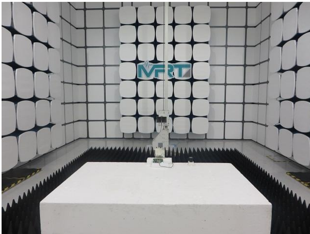
Description: Radiated Emission Test Setup for 18GHz ~ 40GHz (Panel Antenna 15dBi)
