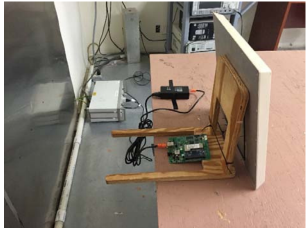
AC Line Conducted Emissions – Rear View
