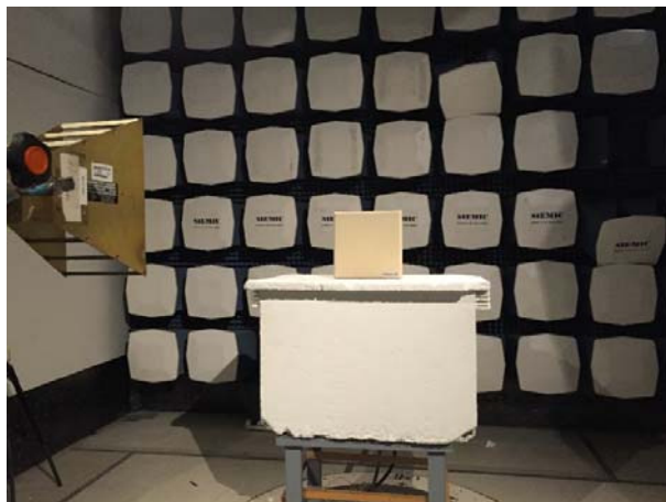
Radiated Emissions (>1GHz) – Front View
