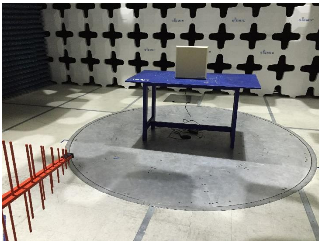
Radiated Emissions (<1GHz) – Front View
