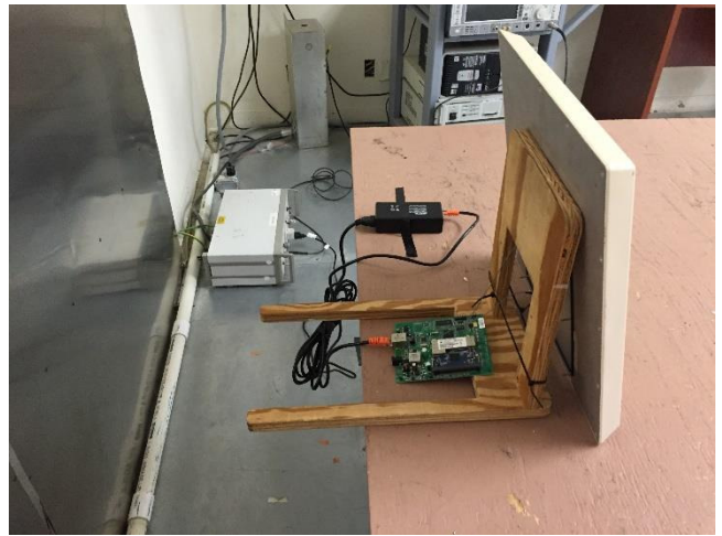
AC Line Conducted Emissions – Rear View
