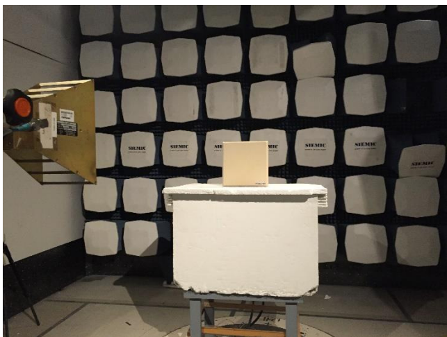
Radiated Emissions (>1GHz) – Front View
