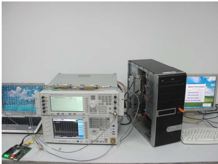
DFS Set-up Photo: Slave and Spectrum Analyzer
