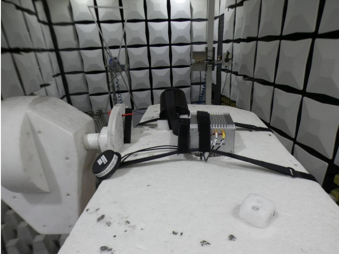
Photo 3: Test setup for radiated measurements FCC Parts 22, 24, 27 and 90, above 1 GHz
