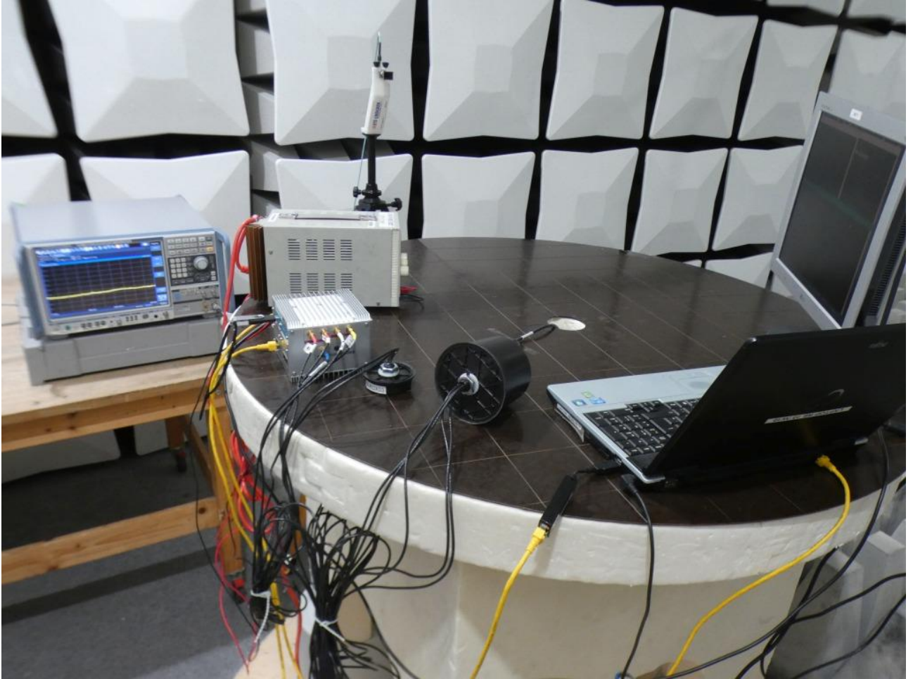
Photo 5: Test setup for radiated measurements FCC15b, 26 GHz – 40 GHz
