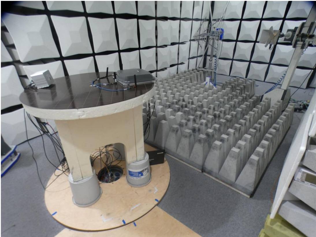
Photo 1: Test setup S01_AA01 for radiated emissions measurements
