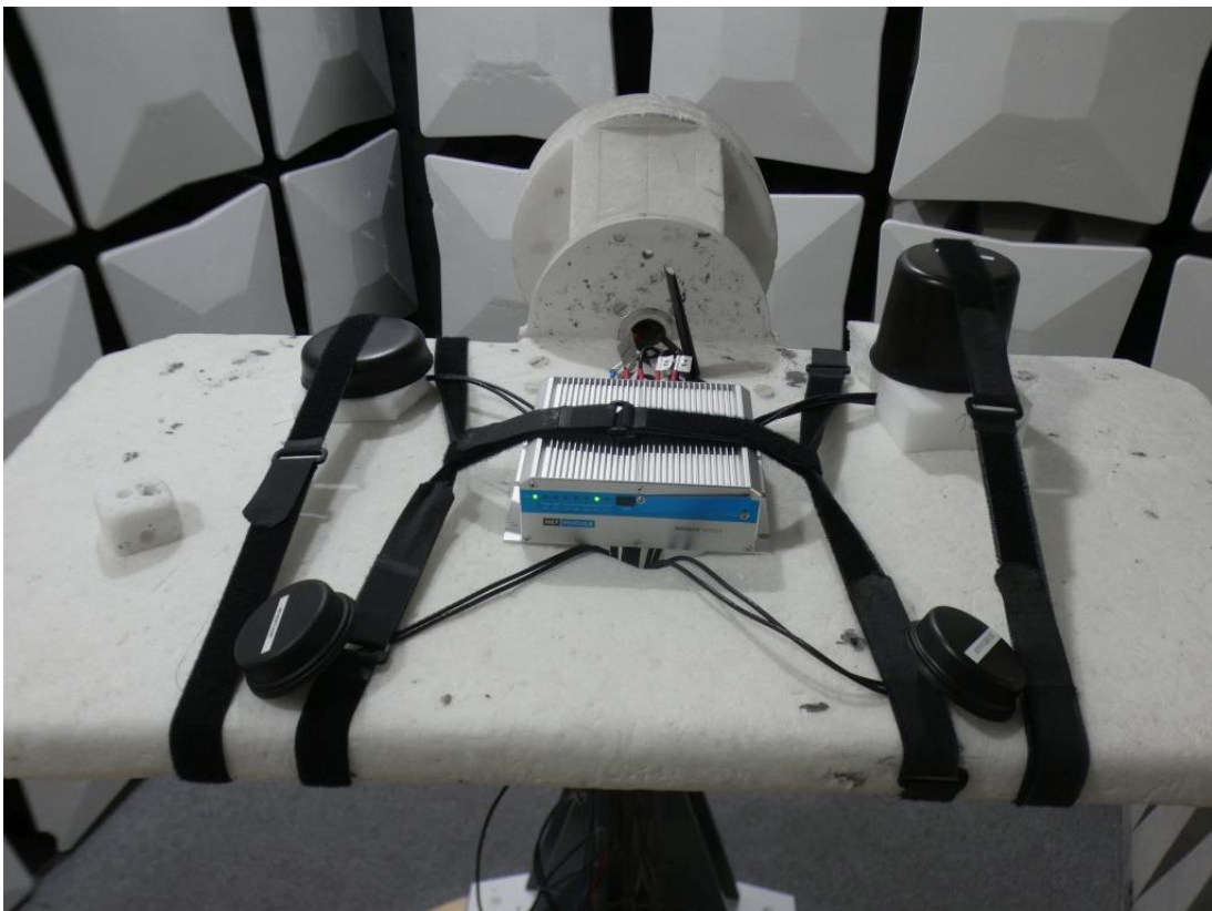
Photo 2: Test setup S01_AA01 for radiated emissions measurements - Detailed view
