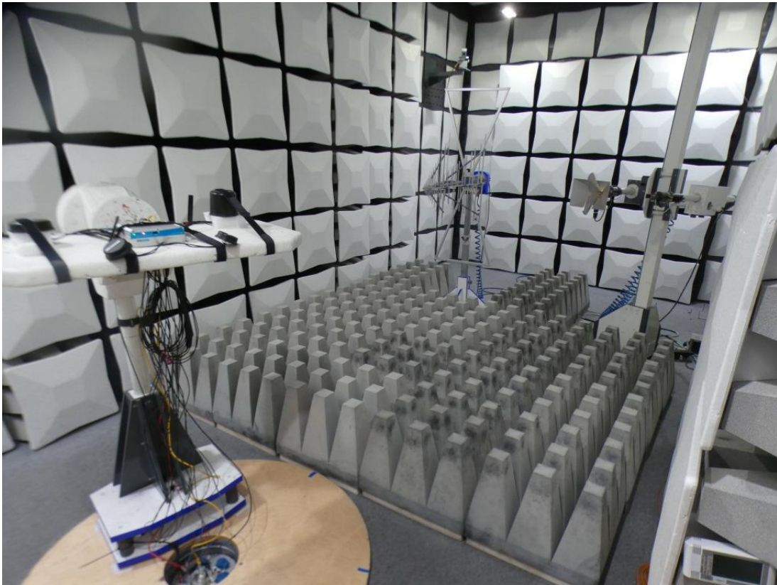
Photo 1: Test setup S01_AA01 for radiated emissions measurements
