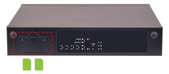
**1.** Loosen the two screws that secure the SIM slot cover and remove the slot cover. With the angled corner facing inward, push the SIM card all the way in until it clicks into place.
