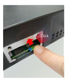
**2.** To remove the SIM card, use your fingertip to push it a little to have the card automatically ejected.
