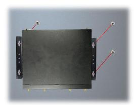
Engage the four screws in the bracket holes, and push the system downwards to lock the screws into position.
