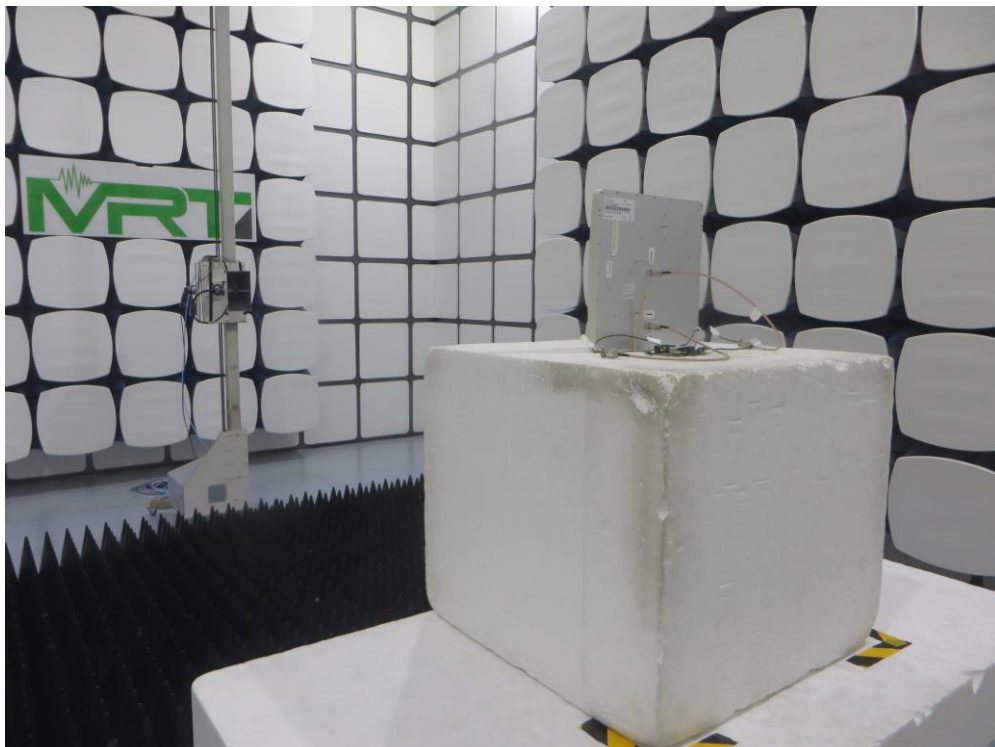
Description: Radiated Emission Test Setup for Above 1GHz (Panel Antenna)
