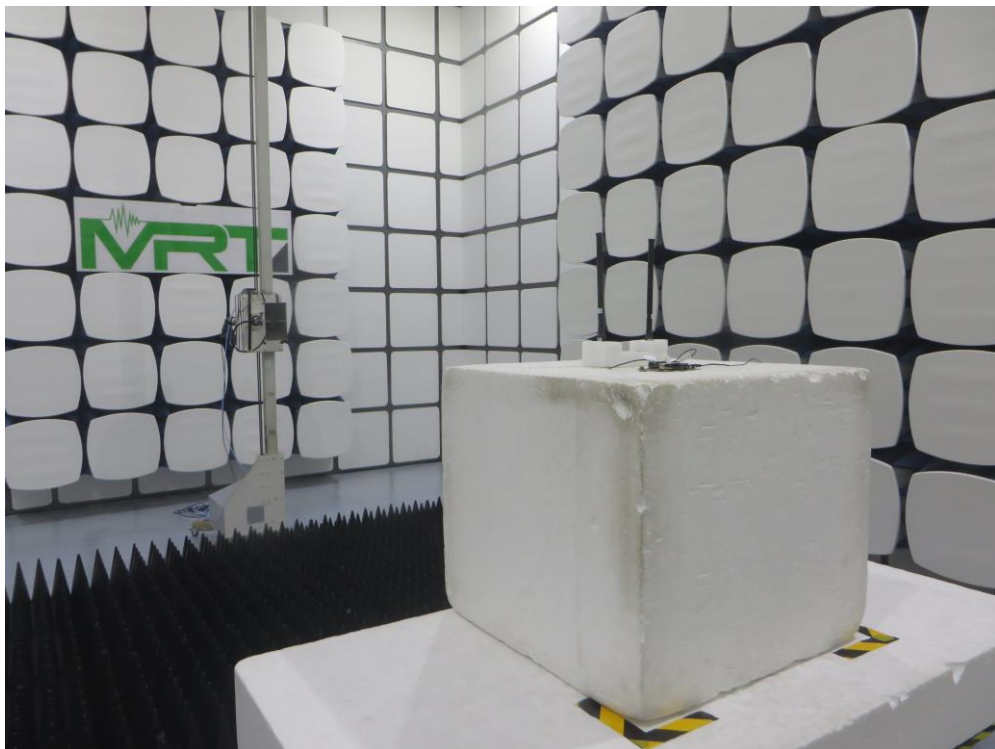
Description: Radiated Emission Test Setup for Above 1GHz (Dipole Antenna)
