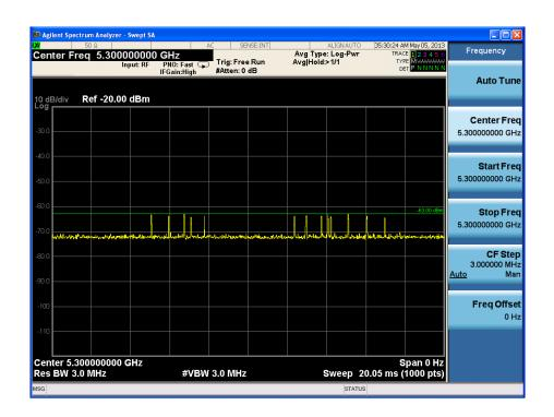
Radar Type 5 Calibration Plot
