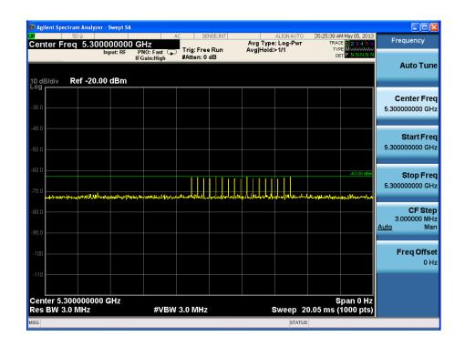
**Radar Type 3 Calibration Plot**
