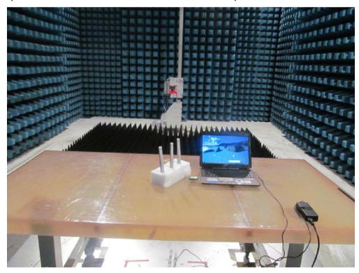
Description: Front View of Radiated Emission Test Setup for Above 18GHz
