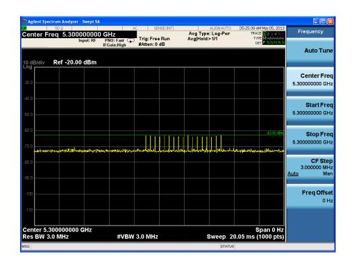
**Radar Type 3 Calibration Plot**
