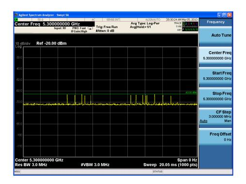
Radar Type 5 Calibration Plot
