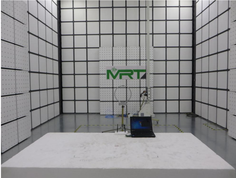
Description: Radiated Emission Test Setup for 9kHz ~ 30MHz with Panel Antenna
