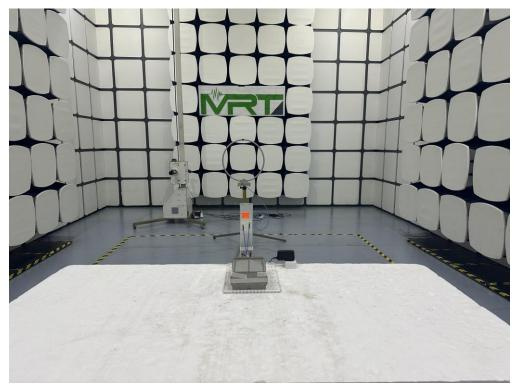
Description: Radiated Spurious Emissions Test Setup for  $30 MHz \sim 1000 MHz$
