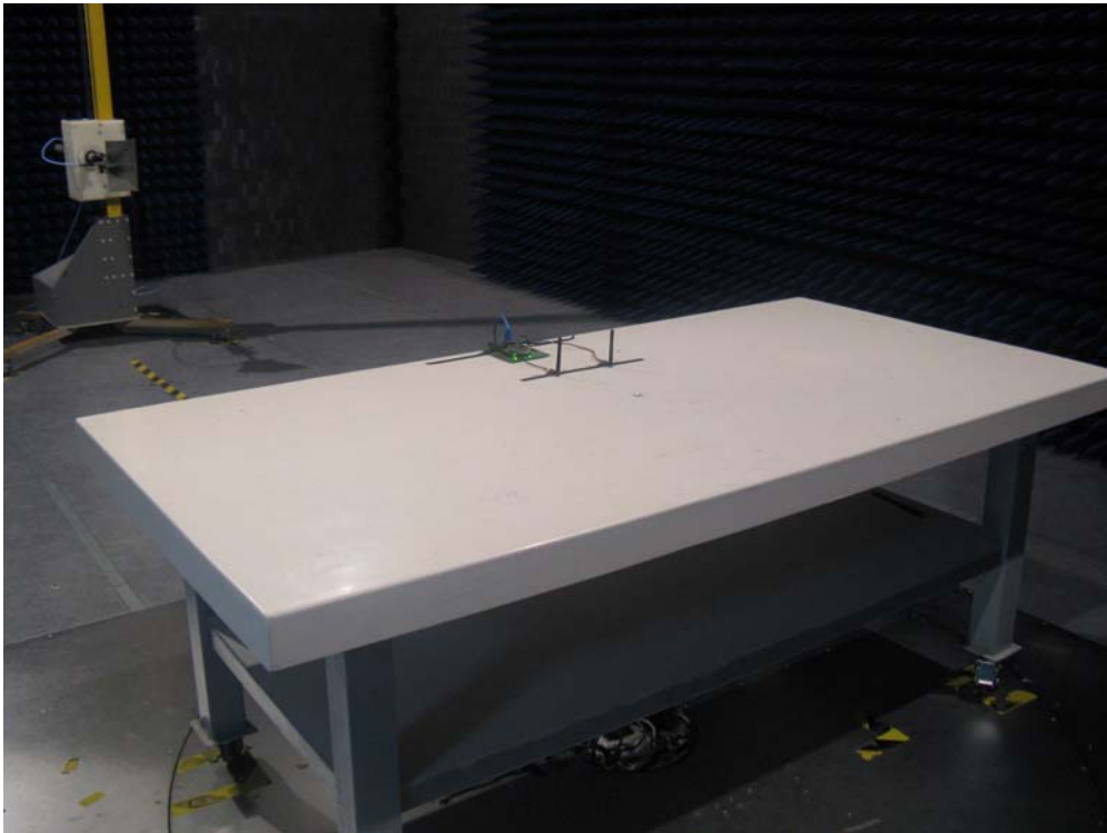
Description : Front View of Radiated Emission Test Setup for Above 1GHz
