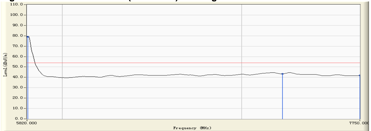
Figure Channel 14: 5840MHz (Horizontal) - Average
