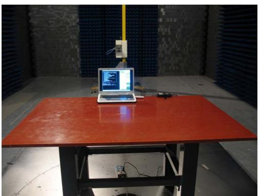
Test Mode: Mode 2: Transmit by 802.11b
