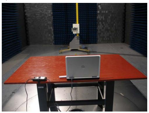
Test Mode: Mode 2: Transmit by 802.11b
