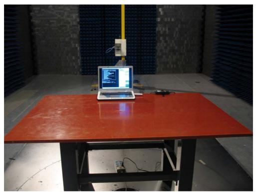
Test Mode: Mode 3: Transmit by 802.11g
