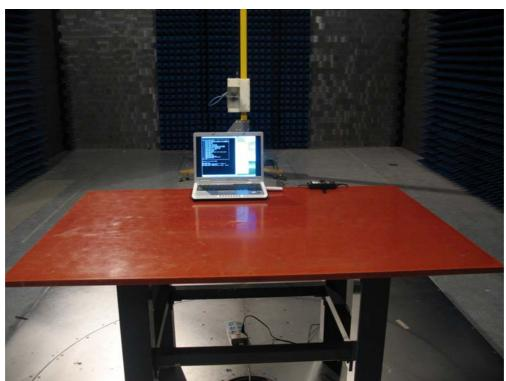
Test Mode: Mode 1: Transmit by 802.11a
