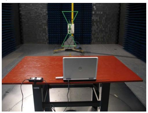
Test Mode: Mode 1: Transmit by 802.11a
