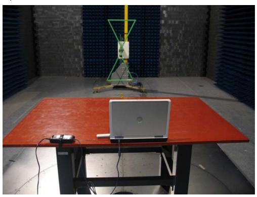
Test Mode: Mode 3: Transmit by 802.11g
