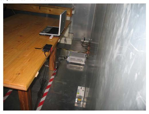
Test Mode: Mode 2: Transmit by 802.11b Description: Front View of Conduction Test
