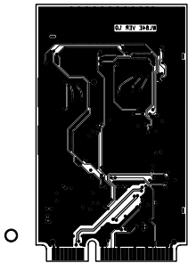
→ 3450 REV 02 BOTTOM FULL RIVER (HK) LTD. WLB4E: 802.11a/b/g/n MINICARD REFERENCE DESIGN VER 1.0
