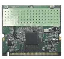
WLM200NX MiniPCI network adapter provides leading 802.11a/b/g/n performance, supporting up to 300Mbps physical data rates and 200Mbps of actual user throughput on both the uplink and downlink. With the dualband design you will enjoy universal connectivity to any 802.11 device through your wireless AP or wireless Router.
