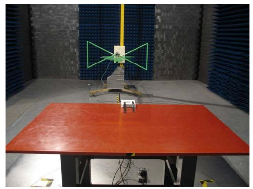
Test Mode : Mode 1: Transmit by 802.11b Description : Back View of Radiated Emission Test Setup for Under 1GHz
