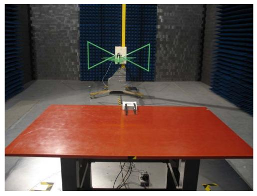
Test Mode: Mode 2: Transmit by 802.11gDescription: Back View of Radiated Emission Test Setup for Under 1GHz
