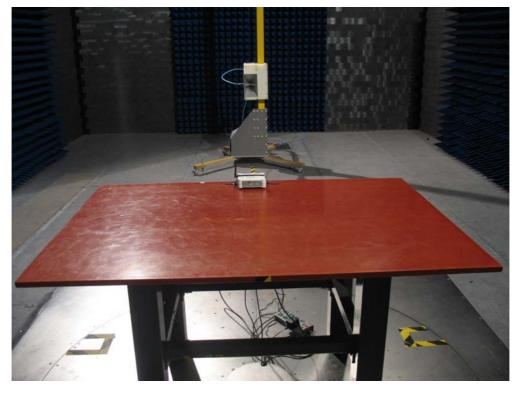
Test Mode: Mode 1: Transmit by 802.11bDescription: Back View of Radiated Emission Test Setup for Above 1GHz
