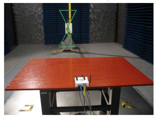
Test Mode: Mode 2: Transmit by 802.11gDescription: Front View of Radiated Emission Test Setup for Above 1GHz
