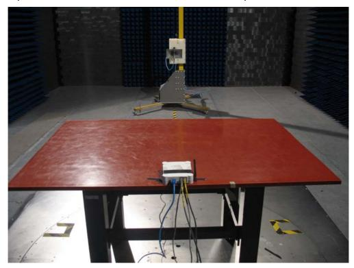
Test Mode: Mode 2: Transmit by 802.11gDescription: Front View of Radiated Emission Test Setup for Under 1GHz
