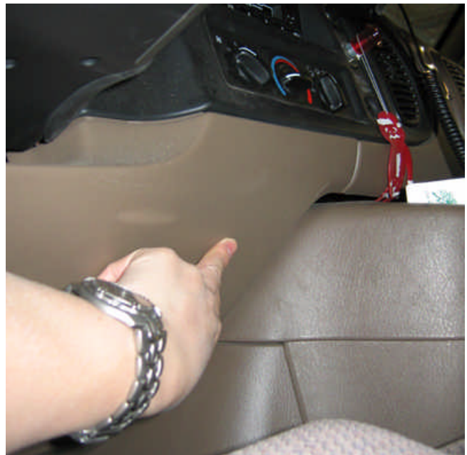
Figure 11: Drill hole for ethernet receptacle
