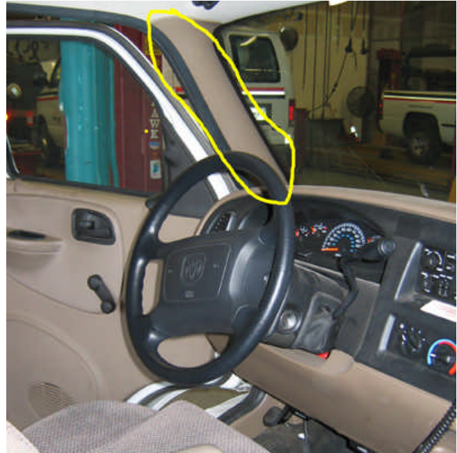
Figure 9: Route cable along driver-side A-pillar
