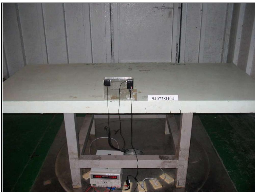
RADIATED EMISSION TEST (Mode 2)
