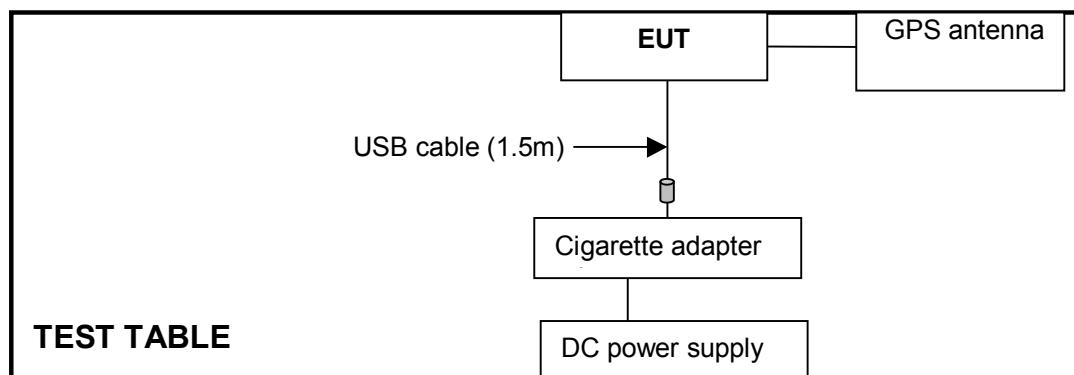
**For AC power conducted emission (Test mode 1) :**
