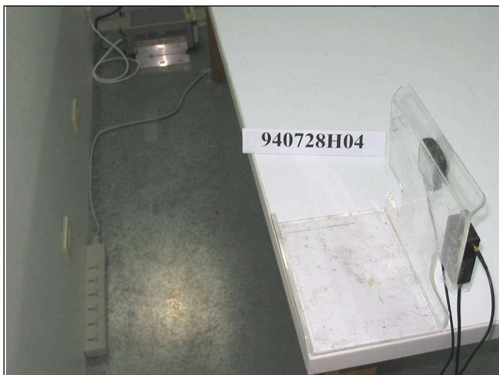
CONDUCTED EMISSION TEST(Mode 2)
