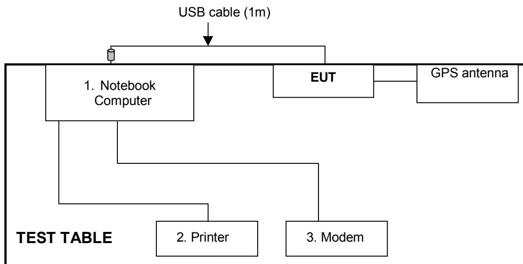
For transmitter radiated emissions (30MHz ~ 1GHz) (Test mode 1) :
