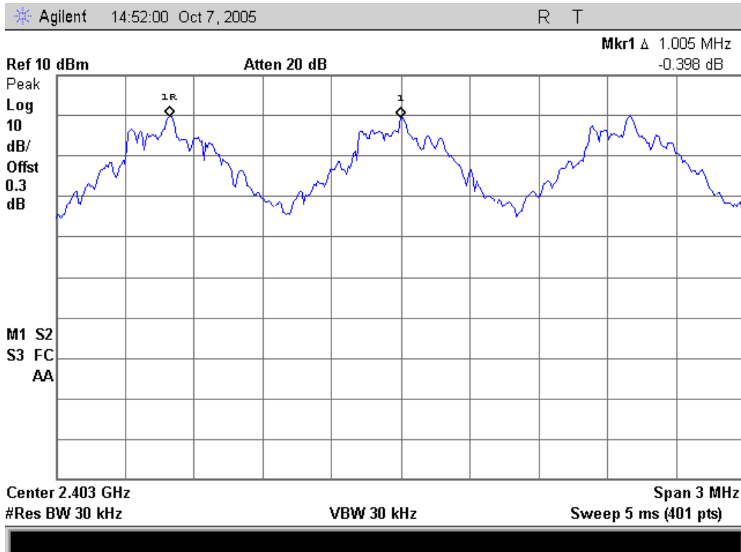
Figure 2. Plot of the Carrier Frequency Separation (Conducted) Lowest Channel (operating at 2402 MHz)
