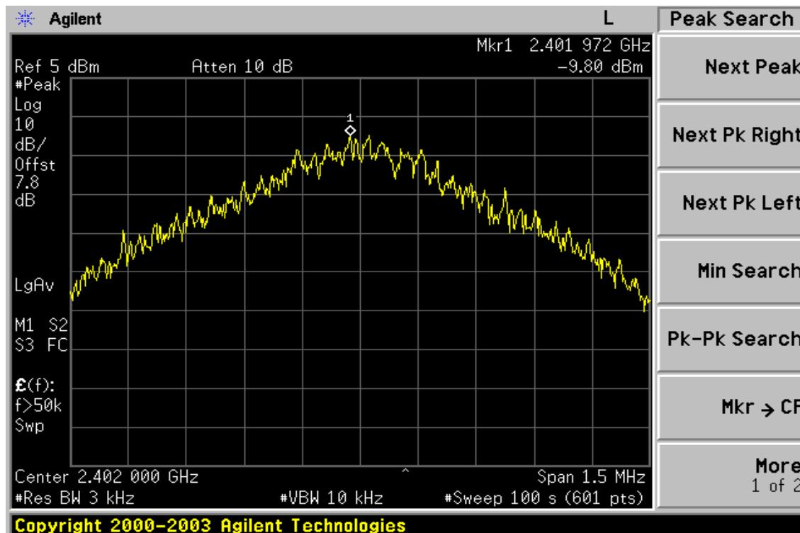
**Power Spectral Density Test Plot (CH-Mid)**
